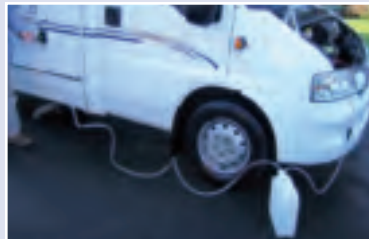
Filling On Board Water Tank
